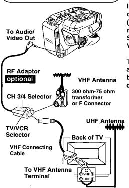
If TV has no VIDEO/AUDIO IN jacks, connect PV-RF16 RF Adaptor (optional). Tune TV to CH 3 or 4 to match RF Adaptor CH 3/4 Selector. Set Adaptor's TV/VCR Selector to VCR for playback.
